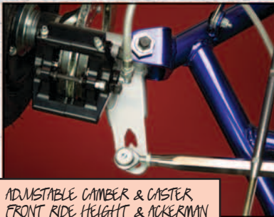
18MM WIDE GROOVED & VENTED BRAKE DISC
