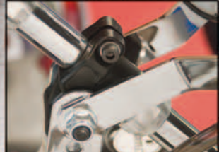
ARROW'S UNIQUE STEERING BUSH WITH CLAMP FOR SIMPLE AND ACCURATE FRONT END ALIGNMENT
