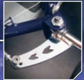
Adjustable camber/caster and front ride height
