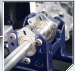
30mm axle supported by three bearings (40mm also available)
