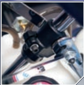
Arrow's unique steering bush with clamp for easy wheel alignment
