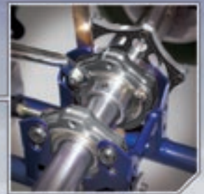
40mm axle supported by three bearings
