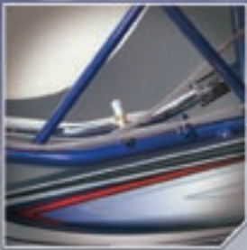
Removable side torsion bar
