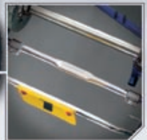
Adjustable/removable rear torsion bar
