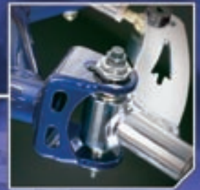
Adjustable camber/caster and ride height
