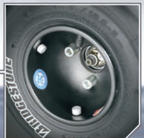
Douglas M-Series black powder-coated magnesium wheels
