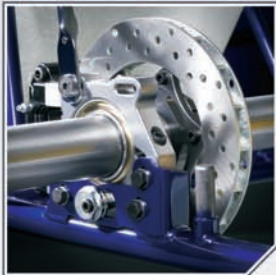
Unique Arrow cam-adjusting rear axle ride height system. Machined billet alloy 4-spot brake caliper mounted directly to bearing flange.
