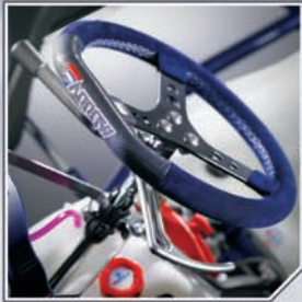
Fully uni-ball jointed clutch lever system, adjustable for position and leverage
