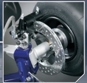
Unique Arrow ventilated front brake discs
