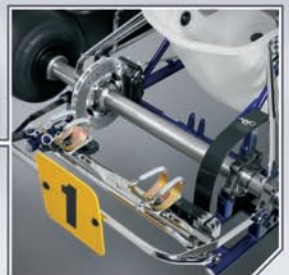
Adjustable/removable rear torsion bar
